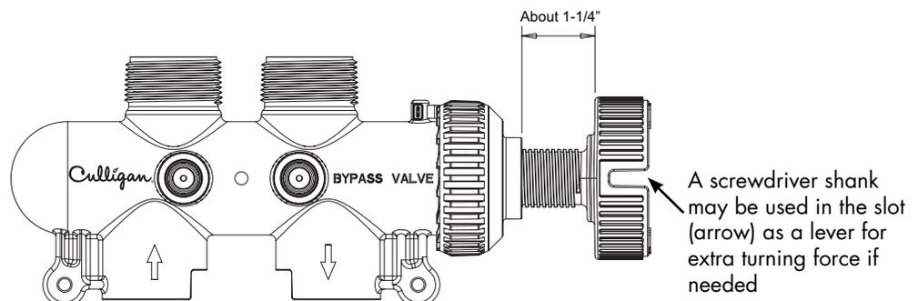
To return to SERVICE, turn the blue knob counter-clockwise (see directional arrow on end of knob) until the knob stops as shown.
