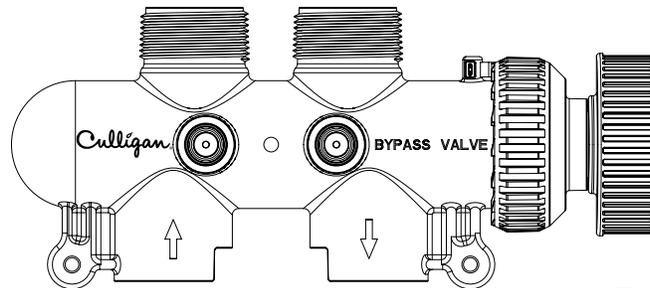
To BYPASS, turn the blue knob clockwise (see directional arrow on end of knob) until the knob stops as shown.
